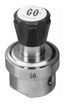
The PR-7LF Series pressure reducing regulator is designed to furnish precise low outlet pressure control to analytical instrumentation. With the combination of the large diaphragm sensing area of the PR-7 Series regulator and the low flow seat assembly of the PR-1 Series pressure regulator, pressure control down to 10 inches of water is easily obtainable.
