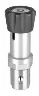
To meet the demands for the safe reduction of inlet pressures up to 10,000 psig, GO Regulator has designed the PR-57 Series regulator. This precision regulator features a piston sensing design which provides the operator with low adjusting torque requirements when setting the outlet pressure. The body is constructed from 316L stainless steel, providing the ultimate in safety and corrosion resistance.
